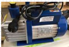
Figure 12: Compressors must not be used for vacuuming
