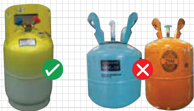
Figure 17: Recovery cylinder (left) and disposable cylinder (middle and right)
