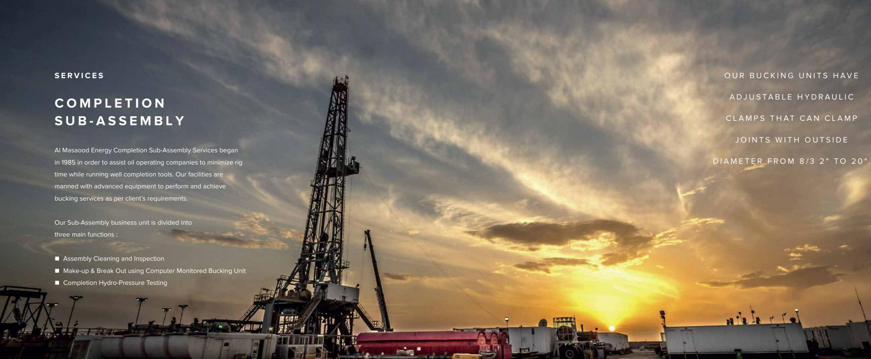
Cleaning is provided with a high-pressure gun and drying air to ensure efficient cleaning to the completion tools. The bucking system is used to make up completions and casing assemblies efficiently. Our bucking units have adjustable hydraulic clamps that can clamp joints with outside diameter from 2 3/8" to 20". Furthermore, provided dies are compatible with any pipe grade from normal carbon-steel to high chromium connection.
