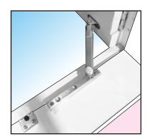
Align The Adjustment Plate Parallel With Window Frame And Fix Screw ( 25 X 6 CSK Head ) In The Second Hole Of The Adjustment Plate As Shown In **Figure 4.**
