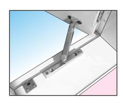
Mark And Screw ( 25 X 6 CSK Head ) The First Hole Of The Adjustment Plate On The Window Frame As Shown In **Figure 3.**
